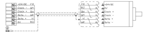
max. cable lenght: 300m cable type: LIYCY 4x2x0.25 + 2x0.5 + shield
